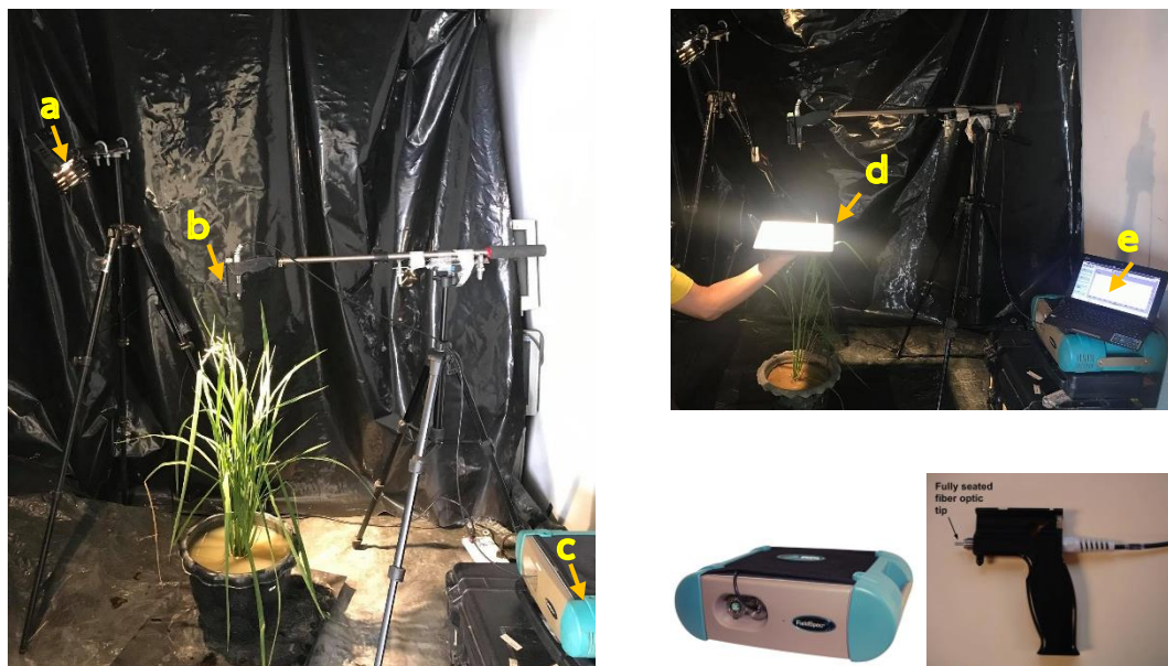
Figure 1 Experimental setup a) Halogen lamp b) Fully assembled pistol grip c) ASD FieldSpec d) White reference panel e) Computer notebook
